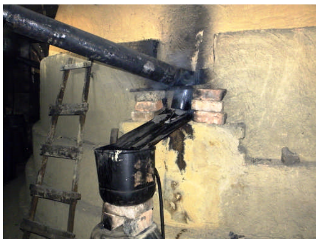
Fig. 1. Smoke from the mangrove charcoal kiln is condensed and collected as wood vinegar
