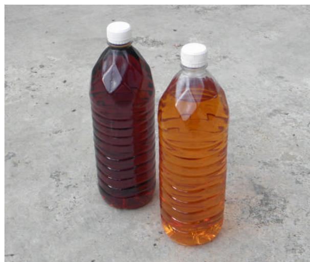
Fig. 2. Non-distilled (left) and distilled (right) mangrove wood vinegar
