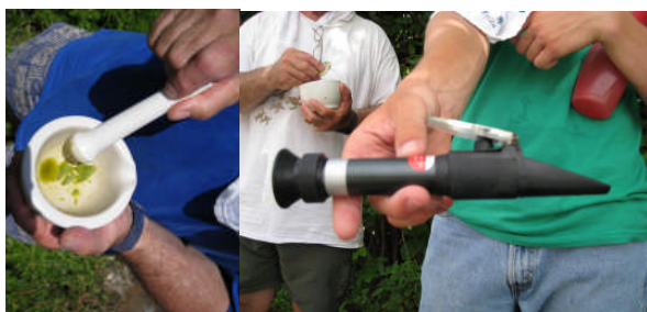
Fig. 2. Grinding mangrove leaf with a mortar and pestle (a) and optical salinity refractometer (Huake Instruments, Model: RHS-10ATC) for reading relative salinity (b)
